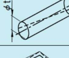
The axis shown by the arrow of the leader line shall be contained within a cylinder of 0.01mm diameter whose axis agrees with the datum axial straight line A.                                                                                                                |
