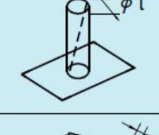
The axis of the cylinder shown by the arrow of the leader line shall be contained within a cylinder of diameter 0.01mm perpendicular to the datum plane A.                                                                                                                    |
