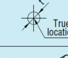
The point shown by the arrow of the leader line shall be contained within a circle of 0.03mm diameter having its center at the true location 60mm and 100mm apart, respectively, from the datum straight line A and from the datum straight line B.                           |
