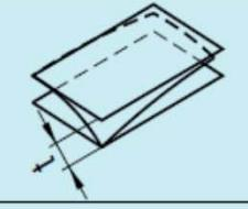
This surface shall be contained between two parallel planes 0.08mm apart.                                                                                                                                                                                                       |
