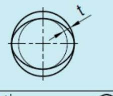
The circumference in any section normal to the axis shall be contained between two concentric circles 0.1mm apart on the same plane.                                                                                                                                            |
