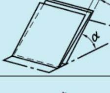
The surface shown by the arrow of the leader line shall be contained between two parallel planes which are inclined at 40° with theoretical exactness to the datum plane A and which are 0.08mm apart from each other in the direction of the arrow of the leader line.       |
