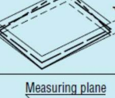
The median surface shown by the arrow of the leader line shall be contained between two parallel planes 0.08mm apart from each other and arranged symmetrically about the datum median plane A.                                                                               |
