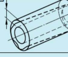
The considered surface shall be contained between two coaxial cylinder surfaces 0.1mm apart.                                                                                                                                                                                   |
