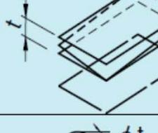
The surface shown by the arrow of the leader line shall be contained between two planes parallel to the datum plane A and 0.01mm apart from each other in the direction of the arrow of the leader line.                                                                      |
