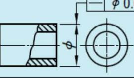
Where a tolerance frame is connected to the dimension showing the diameter of a cylinder, the axis of the cylinder shall be contained a cylinder of 0.08mm diameter.                        |
