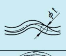
In any cross-section parallel to the projection plane the considered profile shall be contained between two lines enveloping circles of 0.04mm in diameter, the centers of which are situated on a surface having the theoretically exact profile.                            |
