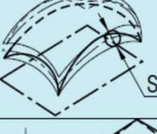
The considered surface shall be contained between two surfaces enveloping the spheres of diameter 0.02mm, the centers of which are situated on a surface having the theoretically exact profile.                                                                              |
